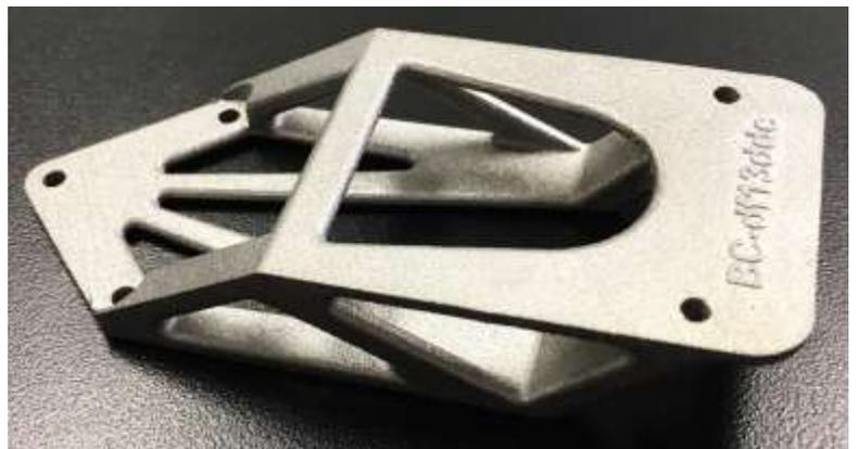
*Photo of a topology optimized 3D printed Ti-6-4 aerospace part employing part build data transmitted and verified using a Cubichain network and embedded hash encrypted serial number. CalRAM integrated the blockchain hash serial number during the printing cycle.*
